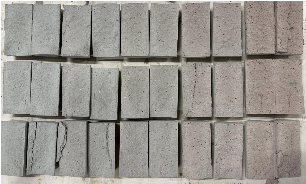
Fig 5.1: Fracture Surface of Laterite Specimen
